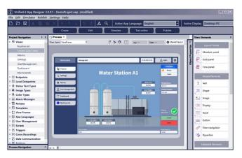
All essential applications—Unified-E App Designer, Unified-E App Manager, and Unified-E App Client—are included at no additional cost. Operator apps are created in the App Designer, installed on the gateway PC, and accessed by operator devices registered with the App Manager. This setup ensures a centralized and secure communication infrastructure between operator devices and endpoints.
